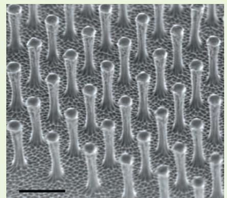
A scanning electron micrograph of micro-fabricated polyimide hairs like those employed on gecko tape. Scale bar is 2 µm. Courtesy AM Geim.
